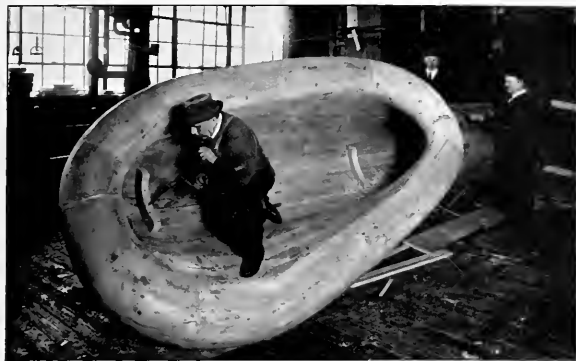
Wooden pattern for the cast steel hawse pipes of the Leviathan in the pattern shop of the Tietjen and Lang plant of the Todd Shipyards Corporation
